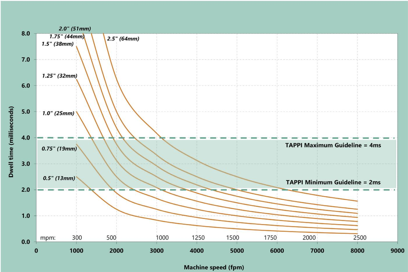
FIGURE 6. TAPPI standards for dwell time over Uhle box slots [modified after 1].
